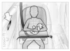
The illustration shows the correct seating position for a child in a child restraint system<sup>\*</sup> with sufficient distance between the child and the side airbag (arrow).
