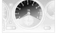
Never allow engine speed to climb until the needle enters the tachometer's red sector.
