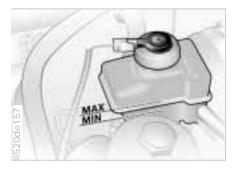
The brake warning lamp comes on and the parking brake has been released: Check the brake fluid level. Fill it to the top mark ("MAX") if necessary.
