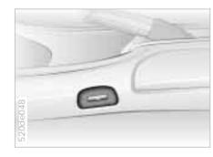
The seat cushion and backrest can be heated when the ignition key is in position 2.
