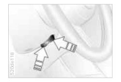
Press the button to move the steering wheel forward or back to suit your selected seating position.
