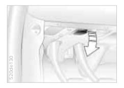
The OBD interface socket for onboard diagnostics is located on the driver's side at the left-hand bottom of the instrument panel and under a cover panel. The cover has the letters "OBD" on it.
