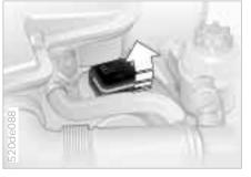
4 Start by connecting the jumper cable from the positive terminal of the support vehicle to the positive terminal connector located in your BMW's engine compartment. The cover of the auxiliary terminal for jump starting is identified by a "+" sign. Refer to the illustration. Remove by pulling the tab (arrow)
