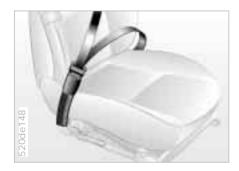
The safety belt tensioner responds to severe frontal collisions by tightening the belt to ensure that occupants remain firmly positioned in their seats. A gas-pressure system retracts the buckle assembly to tension the shoulder and lap belts within fractions of a second. This reduces the tendency to slide under the lap belt.
