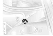
5 Then connect the negative terminals. Attach the cable to either the support vehicle's negative battery terminal (-), or to a suitable ground on its engine or bodywork. Then connect the other end of the cable to a ground on the engine or on the bodywork of the vehicle that is to be started. This is a special nut that is provided on your BMW (refer to the illustration)
