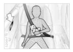
The illustration shows the correct seating position for an older child wearing a safety belt with sufficient distance between child and the side airbag (arrow).
