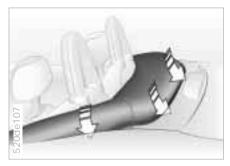
3 Circling it around, push the cover under the rear edge of the convertible top well. Lightly pounding on the cover makes it easier to attach properly
