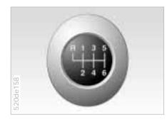
Every time you shift gears, always depress the clutch pedal all the way down, pushing the gear lever into the desired position.
