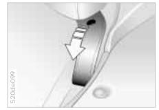
The strap for the belt guide can be opened: release the push button.
